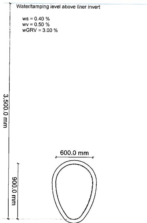
Global imperfection according A 143-2 is understood as an increase (wgrv/10) of the entered local deformation.
