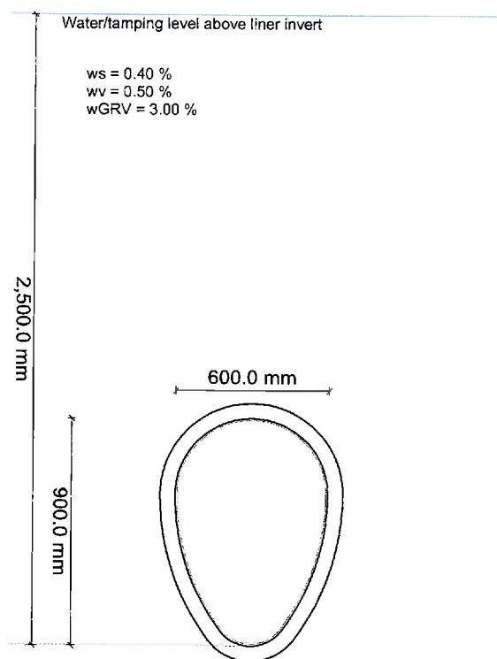
Global imperfection according A 143-2 is understood as an increase (wgrv/10) of the entered local deformation.
