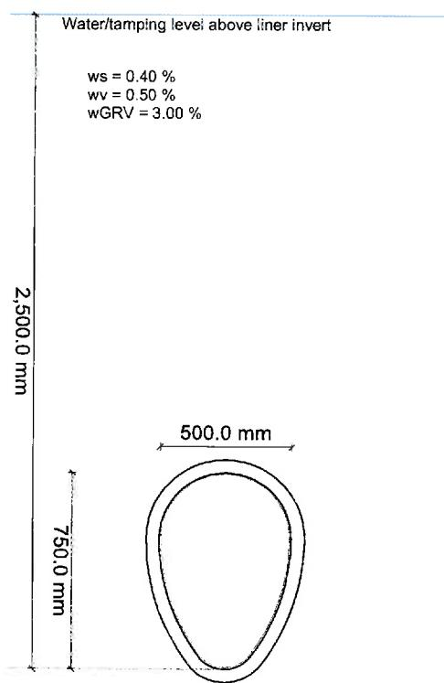
Global imperfection according A 143-2 is understood as an increase (wgrv/10) of the entered local deformation.
