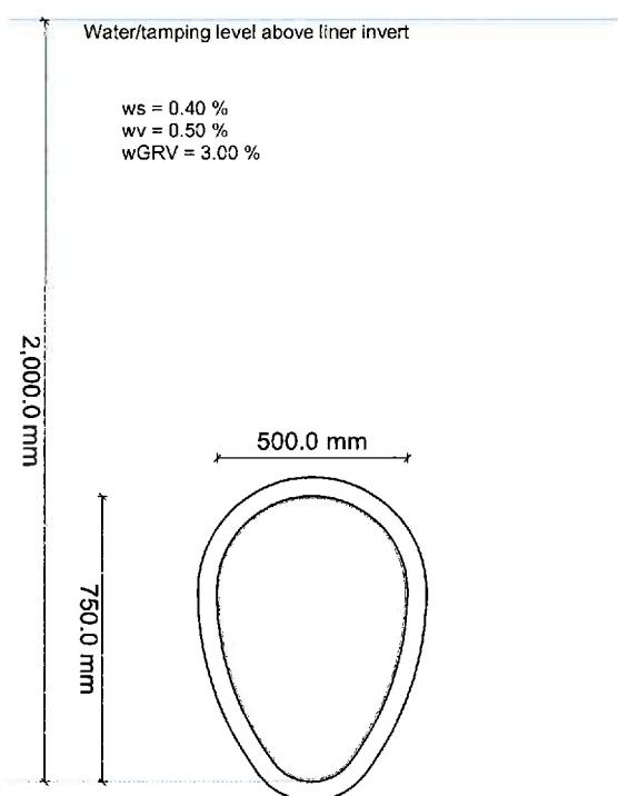
Global imperfection according A 143-2 is understood as an increase (wgrv/10) of the entered local deformation.
